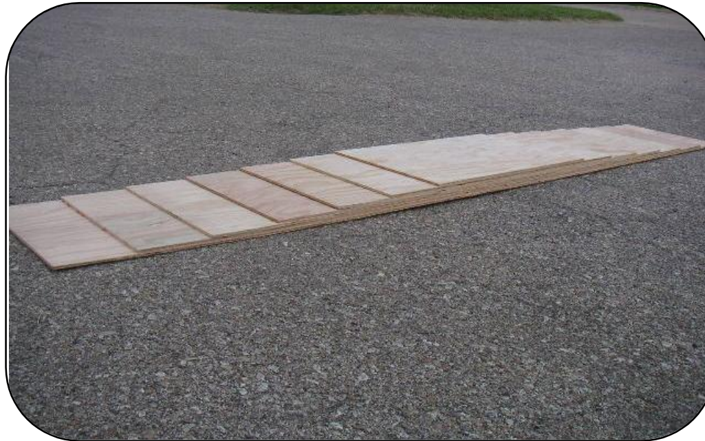
Figure 1: Artificial Bump for Testing Profiling System Accuracy in Detecting Localized Roughness
