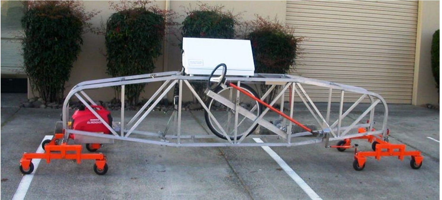
▲ California-Style Computerized Profilograph for Bridge Testing-
