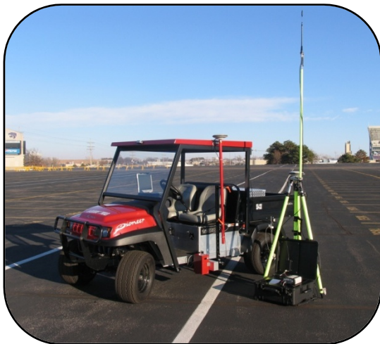
GPS/RTK System Available as a Mobile Surveying Device
