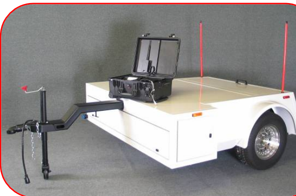
Professionally Engineered Air-Ride Trailer With Independently Suspended Wheels
