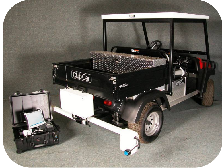
▲ Portable System Configures as a Lightweight Profiler ▲
