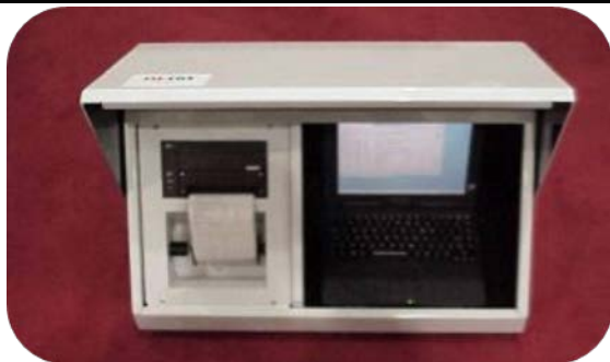
▲ Detachable Operator Housing with AC/DC Power Supplies ▲
