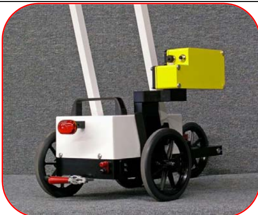
▲ Texture Measurement With Optional Line Scan Laser
