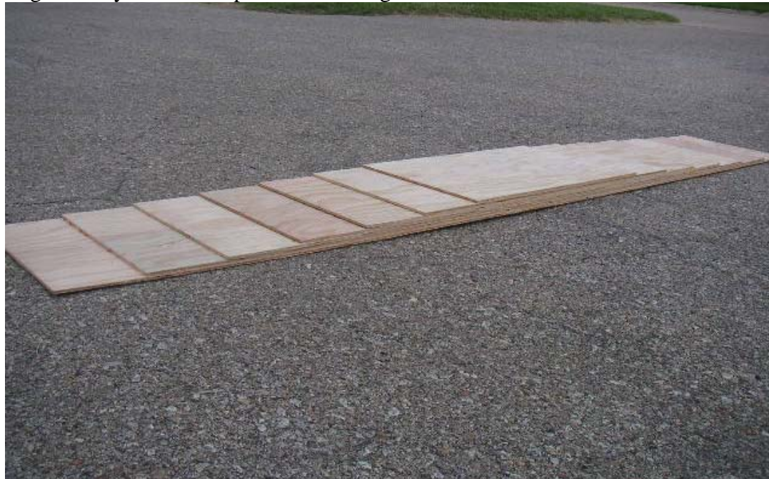
Figure 2: Artificial Bump for Testing Profiling System Accuracy in
