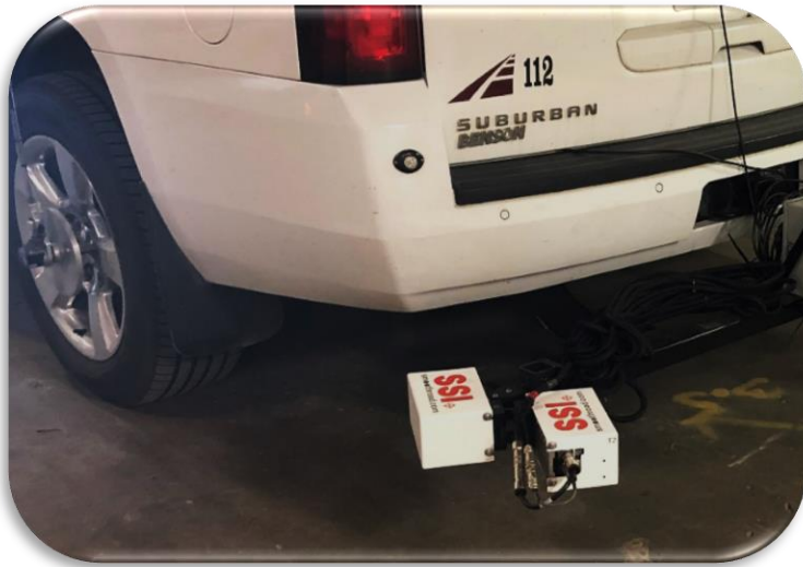
▲ CS9300 Front/Rear Mount Zero-Speed Configuration ▲
