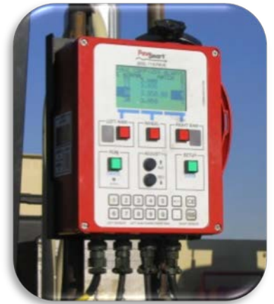
Variable Depth Mill & Paver Control for Smoothness
