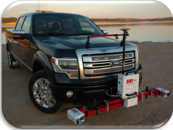
CS9350 Profiler for Surveying and Smoothness Testing
