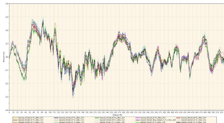
FIGURE 3: Zero Speed Profiler with Vehicle Stoppage vs. Certified IP Operated at Constant Speed
