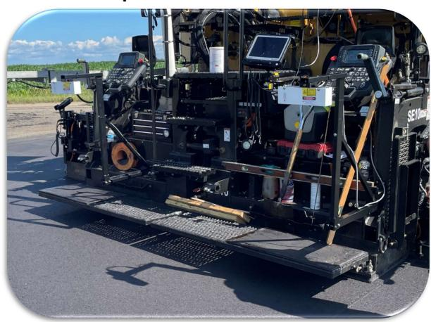
▲ Installs on Pavement Lay-Down Equipment for Real Time Smoothness Testing ▲
