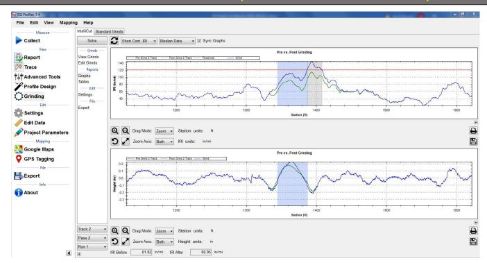
▲ Load Existing Profile Data and Quickly Determine Grind Locations for IRI/MRI/ALR Thresholds ▲
